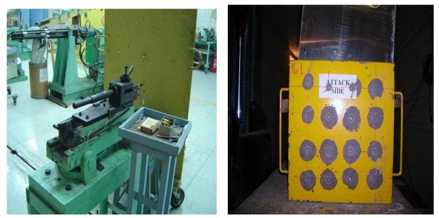
Booths resist .50 cal (12,7\*99mm) Ball **in excess of the requirements of NIJ** (National Institute of Justice) level IV ballistic protection, NATO B7 and EN1063
